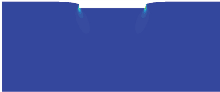
Fig. 24. Strain distribution at a macro scale after conventional forging on 0.8mm depth (scale is shown in figure 23).
