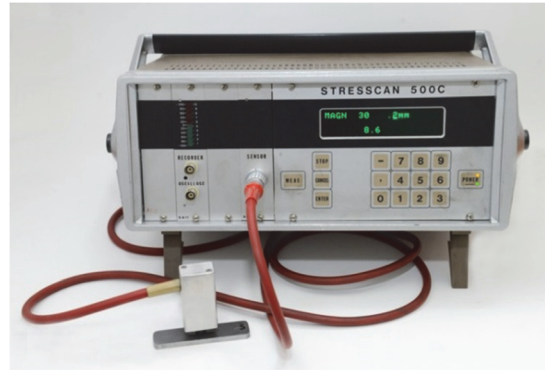
Fig. 2. STRESSCAN 500C apparatus for the stress measurement by magnetic Barkhausen noise method.
