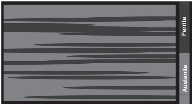
Fig. 8. Distribution of plates of over-saturated ferrite in austenite.
