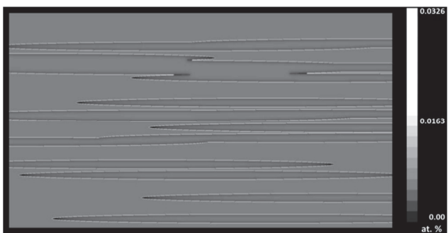
Fig. 9. Carbon distribution of concentration after 350 min.
