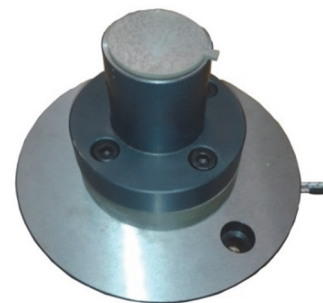
Fig. 2. Experimental setup where the positioning of the workpiece on the lower die can be observed.
