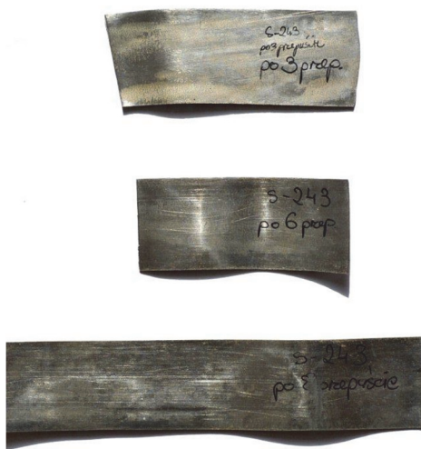
Fig. 4. Example of S243 samples cold rolled after 3 rd , 6 th and 8 th pass.
