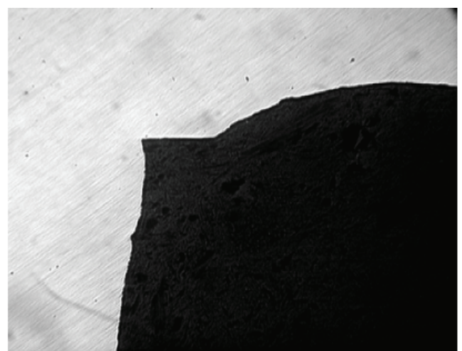
Fig. 3. Faulty shape of the transition radius between the head and the bolt.
