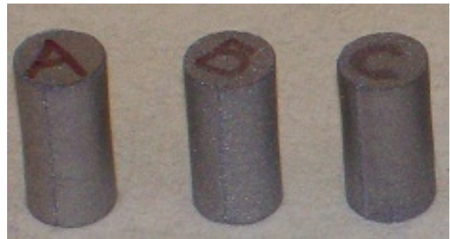
Fig. 2. Ti foam samples for uniaxial compression.
