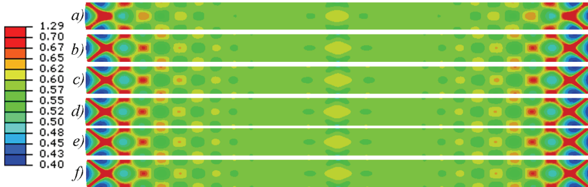
Fig. 8. Equivalent strain distribution for macro models with a different mesh density after channel die test. The density of the FE mesh was selected to obtain expected data transfer nodes between macro and micro scale: a) 2, b) 4, c) 6, d) 11, e) 21, f) 41, respectively (see Figure 5).
