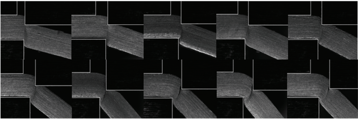
Fig. 6. Set of experimental results for different clearance (0.035-0.485 mm), monitored up to fracture.
