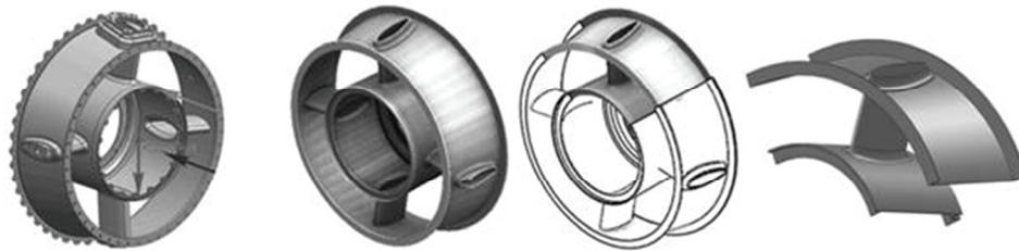
Fig. 1. A simplified model of the geometry of the power turbine casing for a PZL-10W engine.
