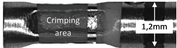
Fig. 9. Contact shape after crimping.
