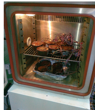
Fig. 8. The experimental equipment: the strain bridge and the climate chamber.
