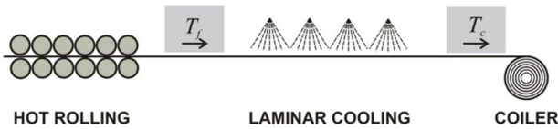
Fig. 2. Schematic illustration of the considered finishing train of the hot strip mill.
