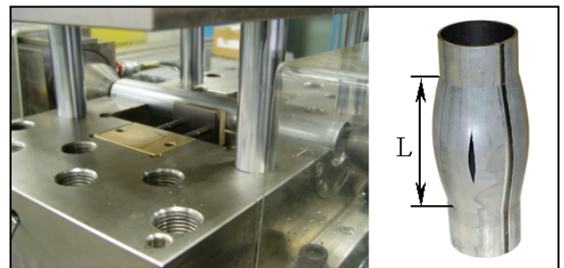
Fig. 2. Bulge-test die and burst tube.
