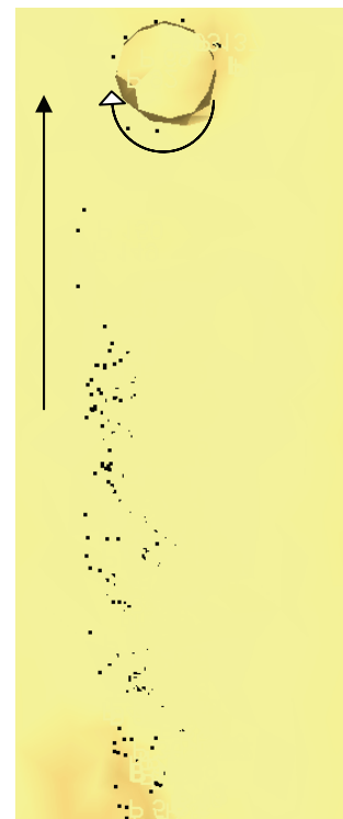
Fig. 9. Top view of the FSW joint – position of the nodes initially placed along the welding line.
