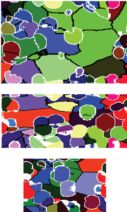
Fig. 5. Microstructure before the 6 th pass, average grain size D = 27 \mu\text{m} . V = 0.00195 \text{ mm}^3 .
