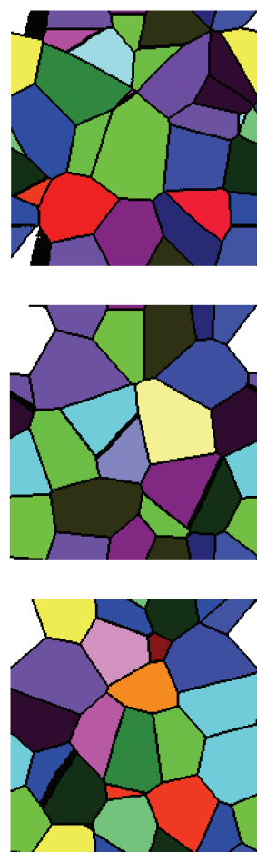
Fig. 3. Initial structure on the planes 0XY, 0XZ and 0YZ respectively, average grain size D = 120 \mu\text{m} . Representative volume V = 0.125 \text{ mm}^3 .
