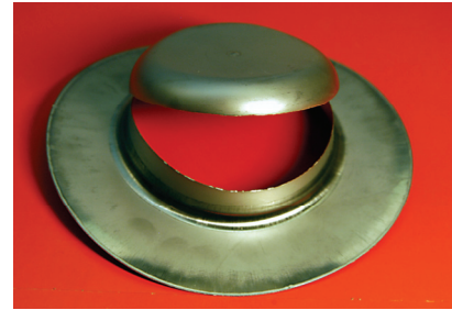
Figure 7. a) Failed steel 304 A after equibiaxial bulging above and b) steel 304 B after deep drawing with cylindrical punch (below).
