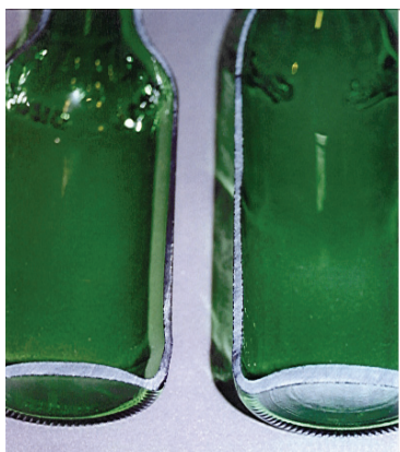
Figure 2. Different glass distributions due to different process conditions
