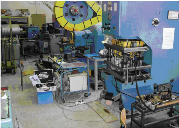
Fig. 11. Remote sheet metal forming process monitoring station
