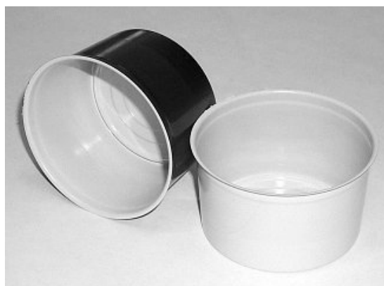
Rys. 1. Puszki z blachy pokrytej polimerem. Fig. 1. Food cans from polymer coated steel sheet.
