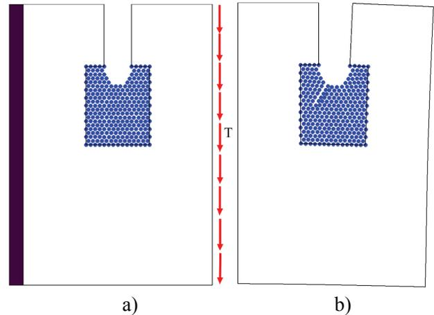
Fig. 6. The plate with the U-notch under the tensile load: a) initial equilibrium without any load, b) equilibrium state of the loaded plate.
