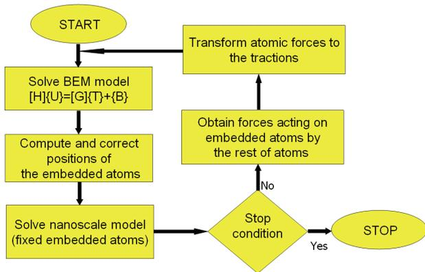
Fig. 5. The algorithm of solving coupled atomistic-BEM model.
