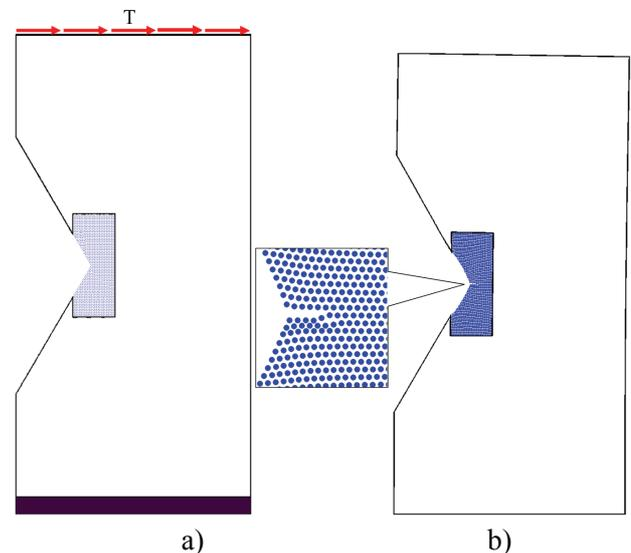
Fig. 7. The plate with V-notch under the tensile load: a) initial equilibrium without load, b) equilibrium state under shear load.
