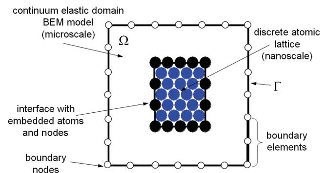
Fig. 4. The coupled BEM-atomic multiscale model.
