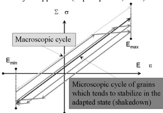
Fig. 4. Macroscopic behavior of the structure and Microscopic behavior of a grain misoriented which undergoes a plastic deformation
