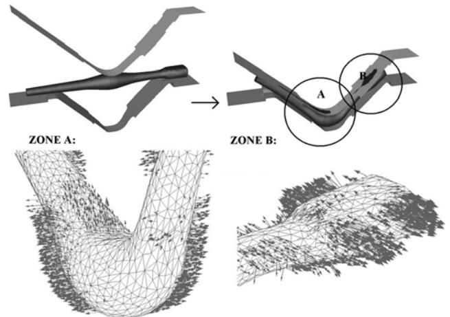
Fig. 2. Flow orientation for a cambering process.
