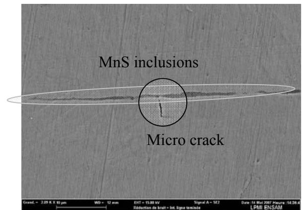
Fig. 7. Cracks are initiated near MnS inclusions (Pessart et al., 2007).
