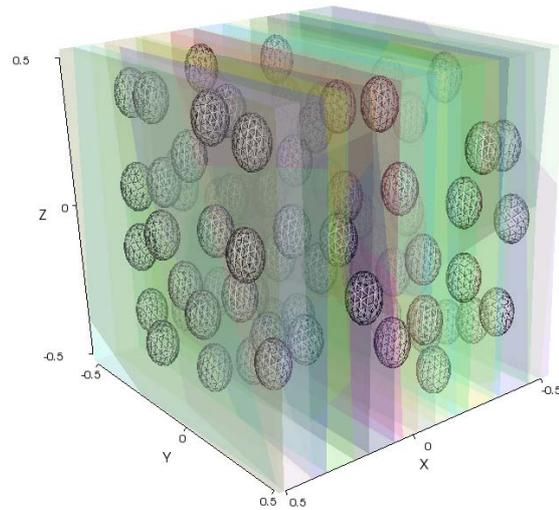
*Fig. 10. Oriented granular structure with 100 inclusions.*
