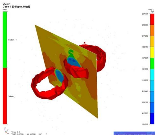
Fig. 11. Stress concentration around two inclusions.
