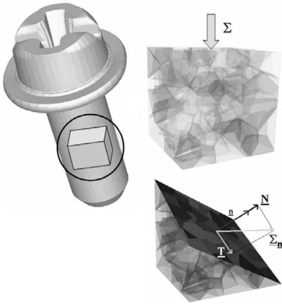
Fig. 3. Schematics of a Representative Elementary Volume (R.E.V.).
