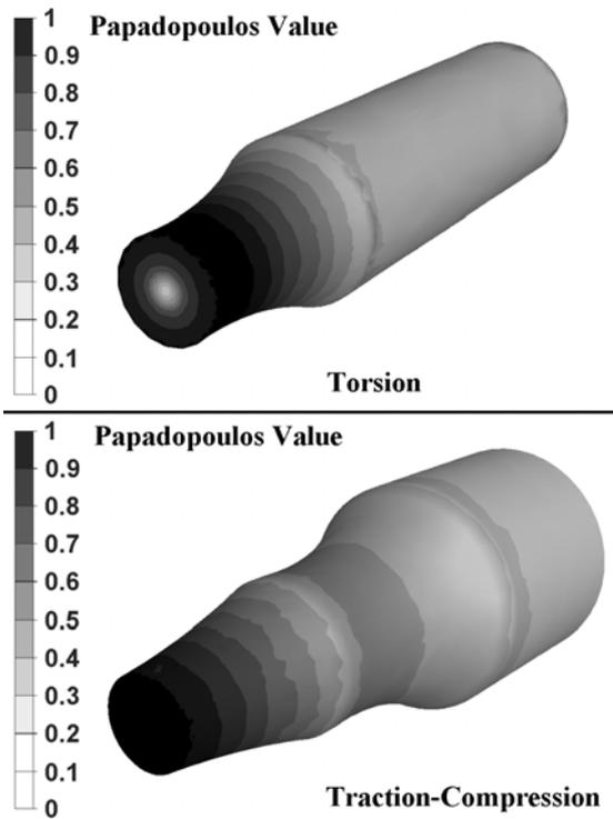
Fig. 6. Normalized Papadopoulos criterion calculated on standardized traction-compression and torsion test specimens.
