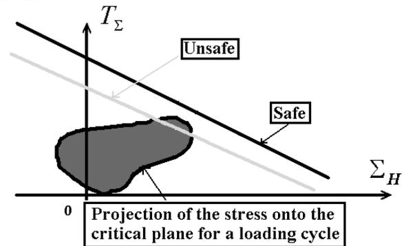
Fig. 5. Threshold domain for a deterministic fatigue criterion.
