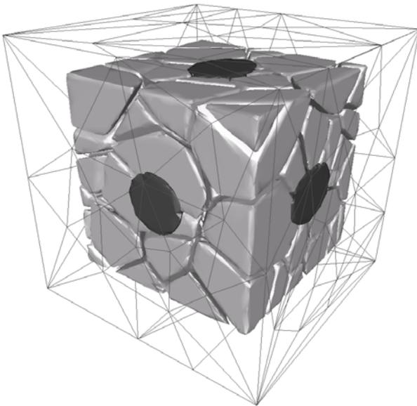
*Fig. 9. Mesh of a microstructure composed of 100 grains and 6 inclusions.*
